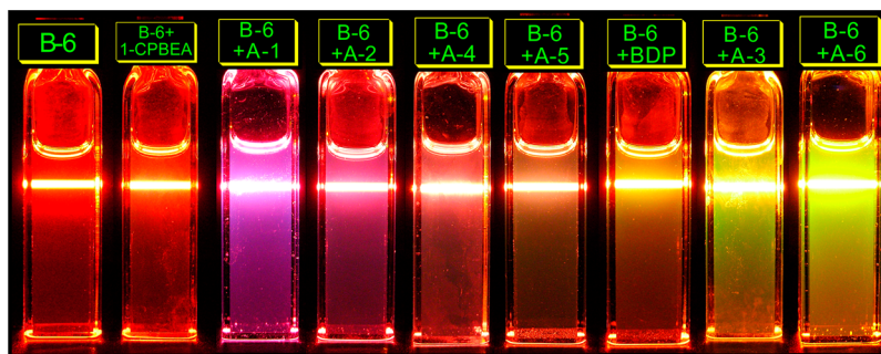
Figure 12. Photographs of the emission of triplet photosensitizer (B-6) alone and the TTA assisted upconversion. Excited with 589 nm laser (4.8 mW). The use of different triplet acceptors is marked. c [B-6] = 2.0 \times 10^{-6} M; c [acceptor] = 4.0 \times 10^{-5} M; in deaerated toluene, 20 °C.
